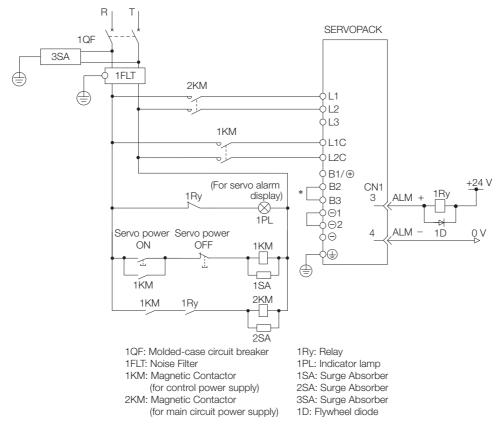
$<sup>\</sup>ast$  You do not have to connect B2 and B3 for the following models: SGD7S-R70A, SGD7S-R90A, SGD7S-1R6A, and SGD7S-2R8A. Do not connect them.
