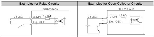
Note: The 24-VDC external power supply capacity must be 50 mA minimum.
