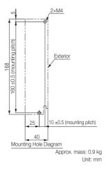
Three-phase, 200 VAC: SGD7S-2R8A; Single-phase, 100 VAC: SGD7S-R70F, -R90F, and -2R1F
