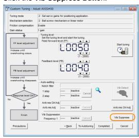
3. Click the Import Button or click ▲ and ▼ Button to manually adjust the set frequency. When you click the Import Button, the residual vibration frequency in the Servomotor is read as the set frequency. (The frequency can be read only when the residual vibration frequency is between 1.0 and 100.0.)
