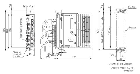
• Three-phase, 200 VAC: SGD7S-3R8A, -5R5A, and -7R6A; Single-phase, 100 VAC: SGD7S-2R8F
