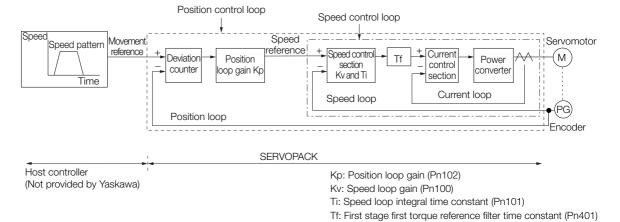
In order to manually tune the servo gains, you must understand the configuration and characteristic of the SERVOPACK and adjust the servo gains individually. In most cases, if you greatly change any one parameter, you must adjust the other parameters again. To check the response characteristic, you must prepare a measuring instrument to monitor the output waveforms from the analog monitor.
