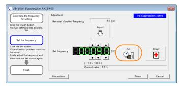
If the vibration is not eliminated, use the  $\triangle$  and  $\blacktriangledown$  Buttons for the set frequency to fine-tune the value and click the **Set** Button again.
