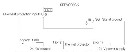
Closed when normal (low temperature) and open when activated (high temperature)
