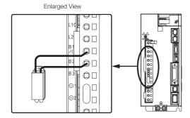
3. Set Pn600 (Regenerative Resistor Capacity) and Pn603 (Regenerative Resistance). Refer to the following section for details on the settings.
