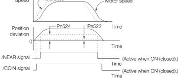
Note: Normally, set Pn524 to a value that is larger than the setting of Pn522 (Positioning Completed Width).
