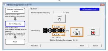
Click the **Reset** Button during adjustment to restore the setting to its original value. The status from before when adjustment was started will be restored.
