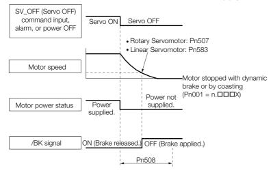
• When the Time Set In Pn508 Elapses after the Power Supply to the Motor Is Stopped
