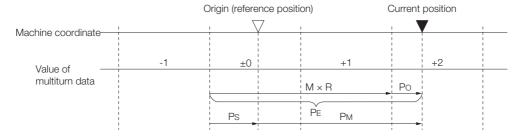
The current position P<sub>M</sub> in the machine coordinate system is calculated as follows:
