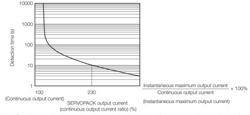
Note: The above overload protection characteristics do not mean that you can perform continuous duty operation with an output of 100% or higher.
