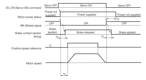
\*1. Rotary Servomotors: The brake delay times for Servomotors with Holding Brakes are given in the following table. The operation delay times in the following table are examples for when the power supply is switched on the DC side. You must evaluate the actual brake delay times on the actual equipment before using the application.
