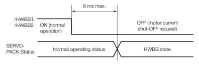
Note: 1. The OFF status is not recognized if the OFF interval of the /HWBB1 or /HWBB2 signal is 0.5 ms or shorter.
