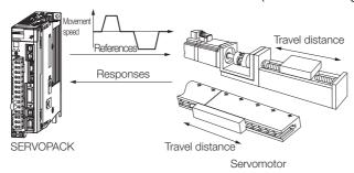
Note: Execute moment of inertia estimation after jogging to a position that ensures a suitable range of motion.
