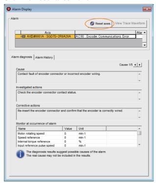
The alarm will be reset, and the alarm display will be cleared.
