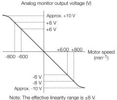
Note: The effective linearity range is  $\pm 8$  V. The resolution is 16 bits.
