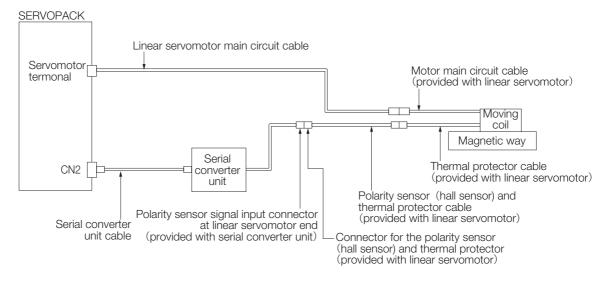
6.14.1 Connecting the Overheat Protection Input (TH) Signal
