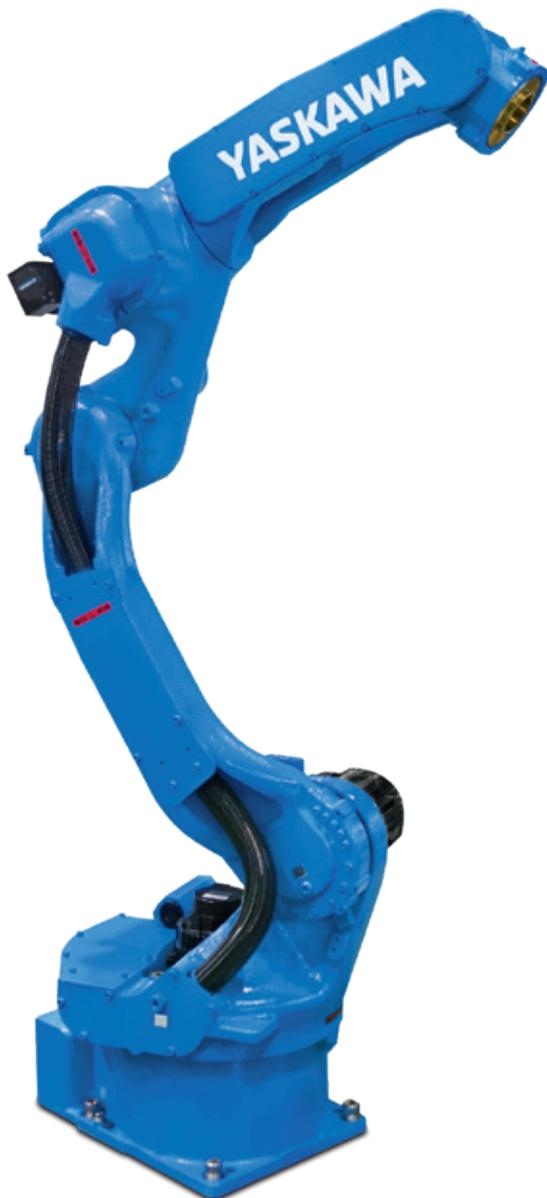
The MOTOMAN GP12 is a fast and precise 6-axis industrial robot with a payload capacity of up to 12 kg. With a reach of 1440 mm and a high repeatability of  $\pm 0.02$  mm, it is ideally suited to assembly tasks, but also universal handling tasks, CNC machine tool tending or packaging. Its streamlined modern industrial design minimizes the space requirements at the installation site.
