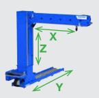
All axes are servo powered and fully synchronised with the robot controller.
