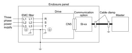
Figure 10.3 Option Installation for CE Compliance: GA500, HV600
