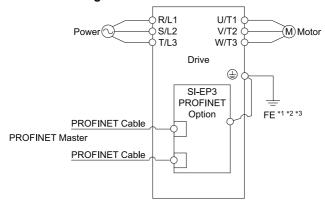
Figure 5.22 Option Connection Diagram
